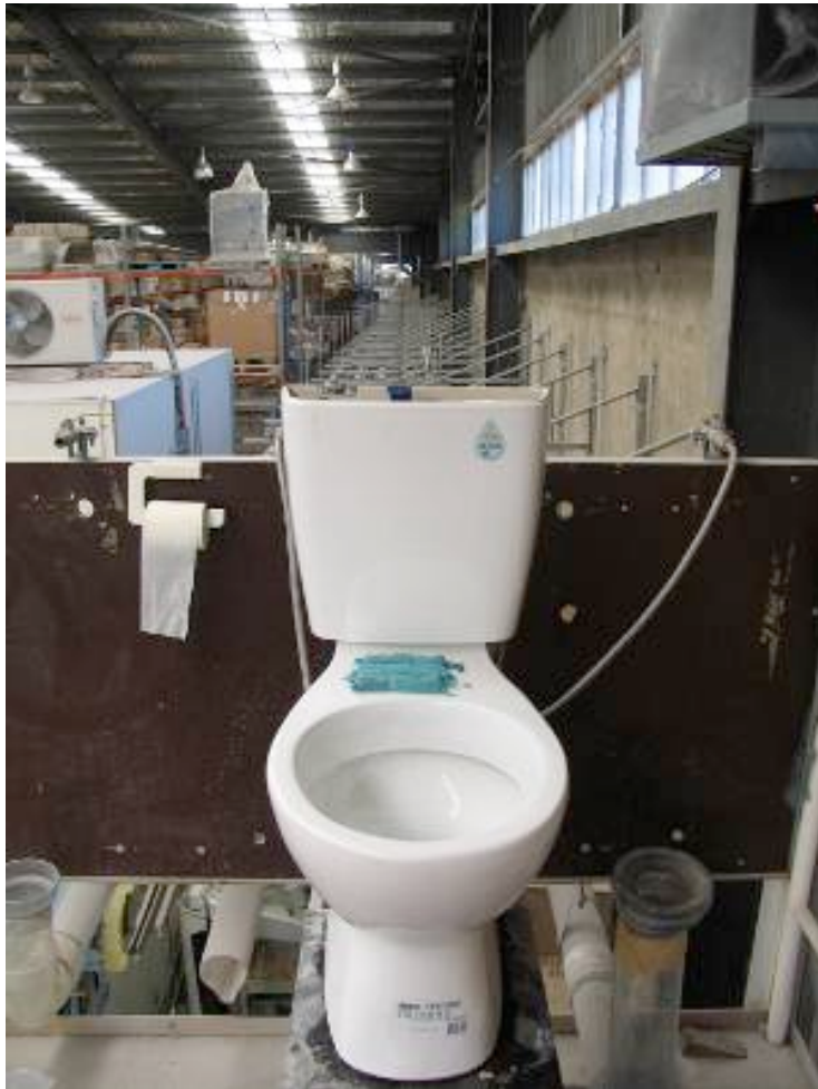
Comprehensive drainline testing conducted on 60m drainline testing rig
