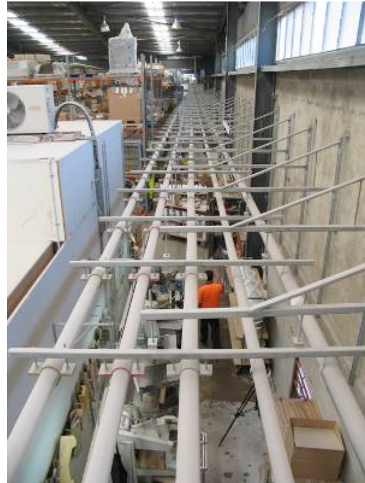
Comprehensive drainline testing conducted on 60m drainline testing rig
