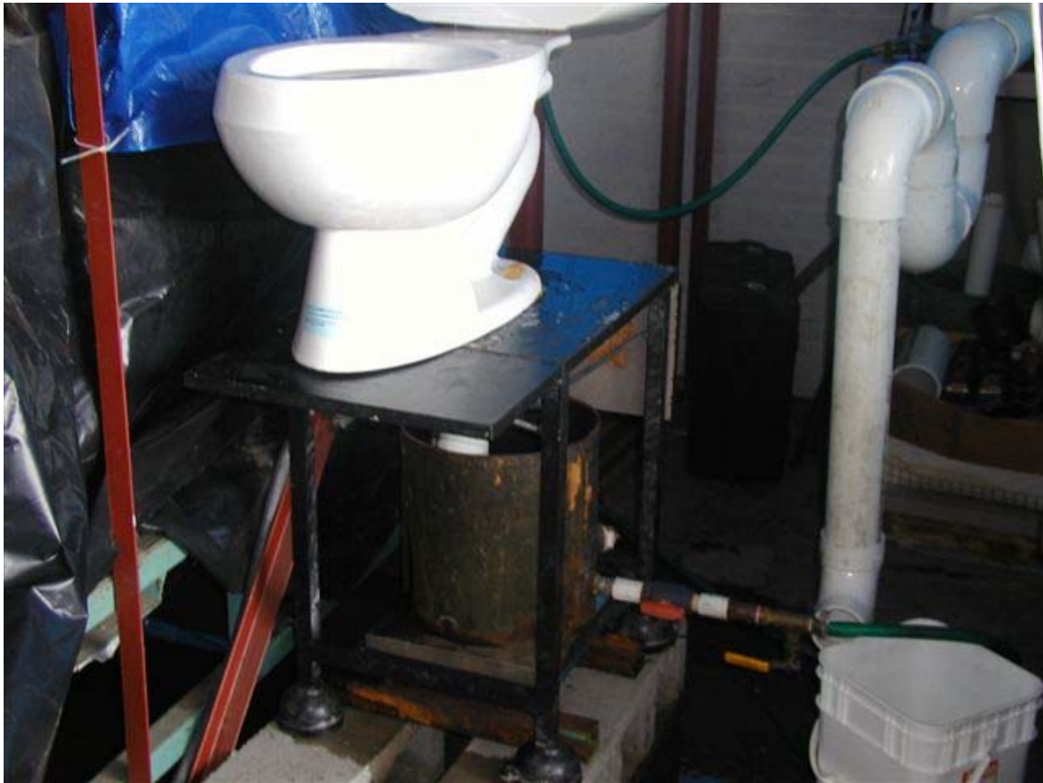
Figure 16: Actual Flush Curve Set-up.
