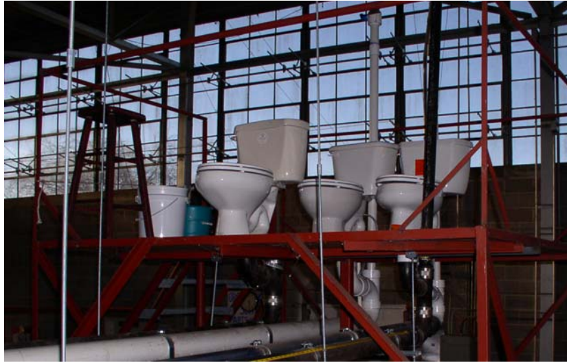
Figure 17: Waste Transport Study Stand and the Four Adjustable Pipe Runs
