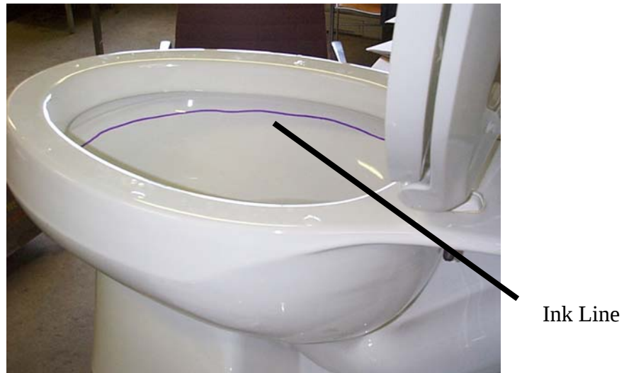
Figure 7: ASME Ink Line Test
