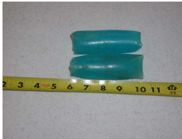
Figure 13: Two Medium Sized Water Wigglers are Utilized to Simulate a Load; Combined Mass of 250 grams
