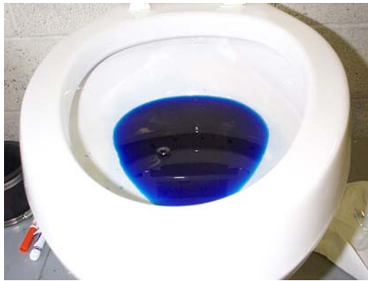
Figure 8: ASME Dye Test
