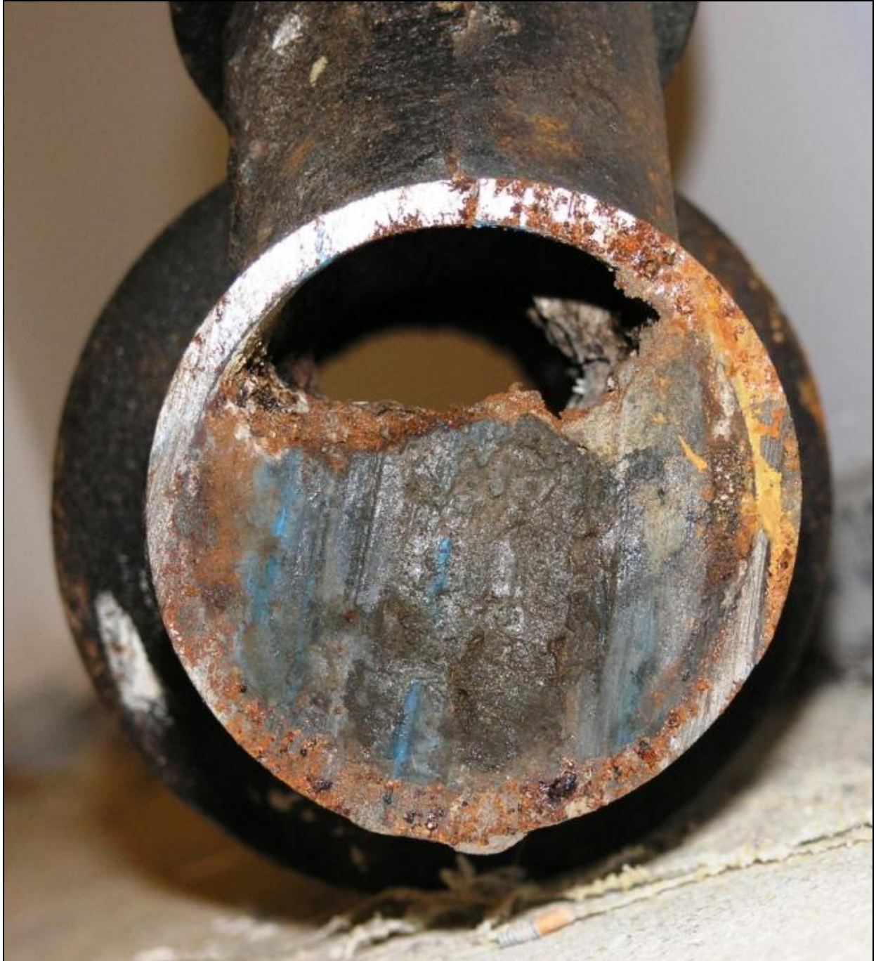
Figure 11. Horizontal fixture run, directly beneath water-flushing urinal at Aquinas College in Grand Rapids, Michigan, removed in 2005 after 12 years of service.
