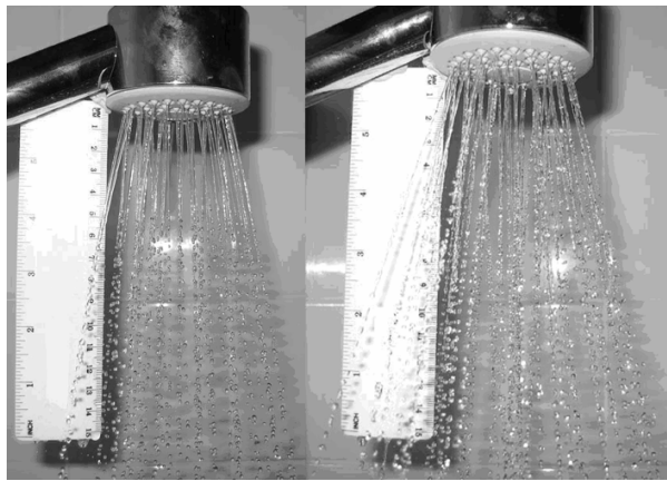
Figure 3: Instantaneous spray form at low (left) and high (right) flow rates
